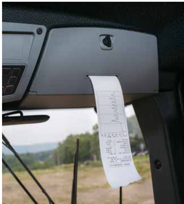
Integrated printer: for documentation of compaction results.
