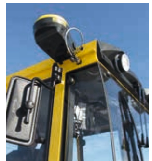
For immediate use anywhere: BOMAG StarFire GPS receiver.
